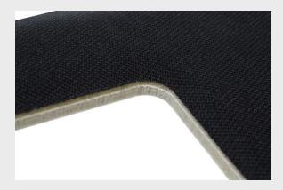
Woodbridge Stratas<sup>™</sup> board package tray composites feature a semi-rigid polyurethane foam core for high sound absorption and reinforcement layers for structural integrity. Our flat substrate boards can be manufactured to virtually any length and width, allowing multiple package trays to be formed at the same time from one super board to decrease cycle times. Our formed package tray shells can be fully assembled and customized with A-surface fabrics and thermoforming services.
