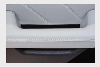
Our thin profile interior foam helps complex, slim-profile interior door armrest components achieve new levels of fit, finish, and comfort. This high-resiliency, high-density foam can be supplied as a stand-alone component or as a finished trimmed assembly. We offer solutions that can eliminate steps in the finishing process including the gluing of foam to substrates with FIP.
