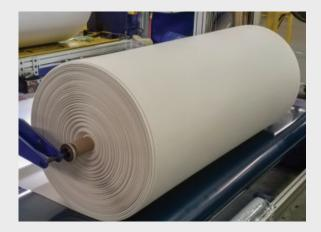
StrataPlush<sup>™</sup> coverstock headliner foams are uniquely designed for a wide range of highly-efficient processes. Formulations are specifically engineered for both wet and dry headliner forming, as well as various other softtrim applications. Woodbridge StrataPlush headliner flexible foam family solutions are engineered to deliver the highly specialized needs of today's laminate foam production environments.
