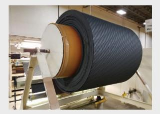
Woodbridge uses flame lamination to create a thin layer of molten polymer to simultaneously bond our AutoBond<sup>™</sup> family of flexible foams to face fabrics and backing materials. Our products are offered for both conventional trim and foam-in-place with a variety of customization options available.
